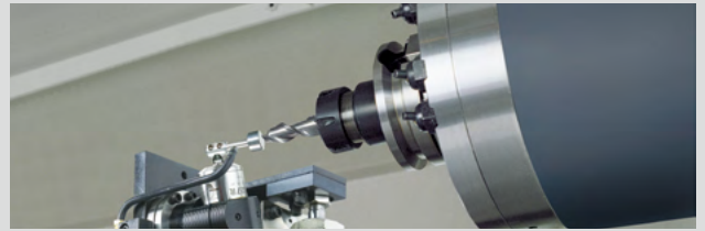
Automatic tool measuring device (TS 27R) option
