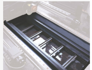
Internal Chip conveyor OPTION (SCRAPER/HINGED)
