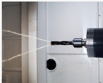
SPINDLE-THROUGH COOLANT (TSC) OPTION
