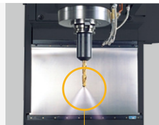
Through-spindle coolant spray system
