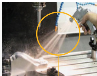
Coolant Gun Coolant gun helps keeping the work environment clean.
